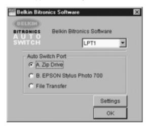
Now, the Bitronics switch will always keep your computer connected to the Zip® Drive. That way, anytime you access it, you will not get any strange errors. Then, when you print to the Ink Jet Printer on Port B (as shown above), the Bitronics switch will switch to Port B temporarily to send the print job, then switch back to Port A to keep communication with the Zip® Drive.
